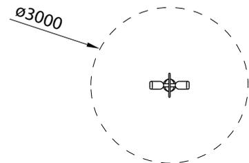
A) Montage in losem Fallschutz
